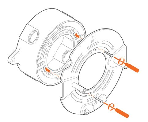
2. Screw the mounting bracket to the adapter plate using the holes in the mounting bracket circle.
